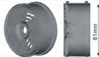
In order to reduce the weight of the rims, the outside diameter is same as the ordinary car, but the inside diameter is 0.079" (2mm) larger. The weight of the rim is only 29g.
