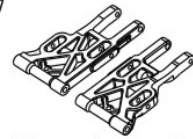
Front Lower Suspensions (Aluminum)
