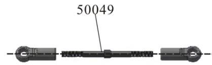
Step22:Steering Linkage Assembly
