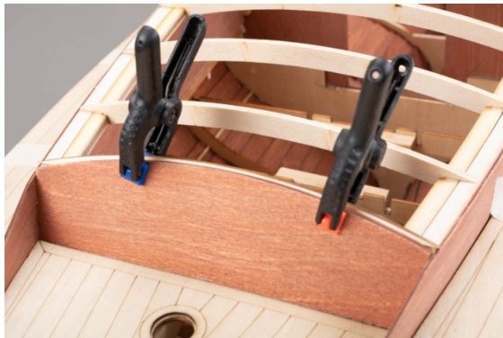
Fig.: Gluing in roof frame 3.17
