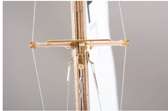
Fig.: spreader, shroud and foresail rigging
