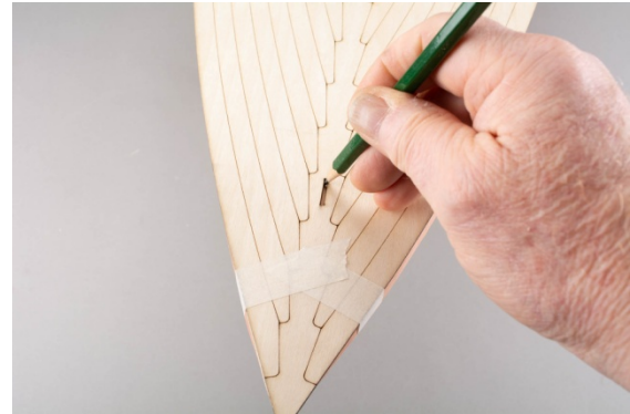
Fig.: Marking the cut-out
