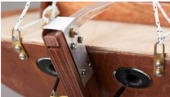
Fig.: Attaching the mounting brackets (shown here at the large RC model)
