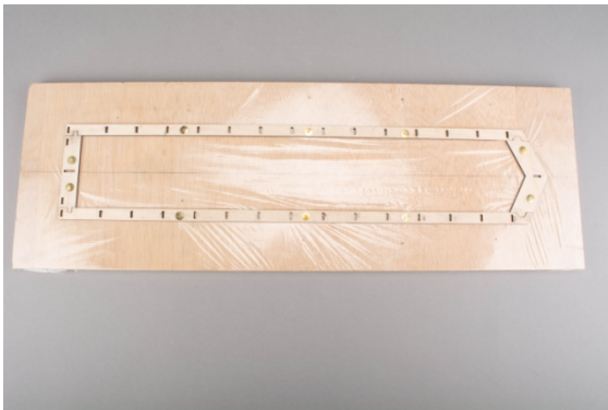
Fig.: Building board with slipway
