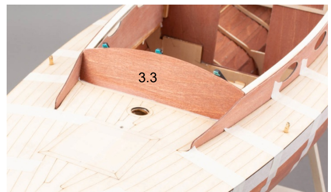
Fig.: Installing the front wall
