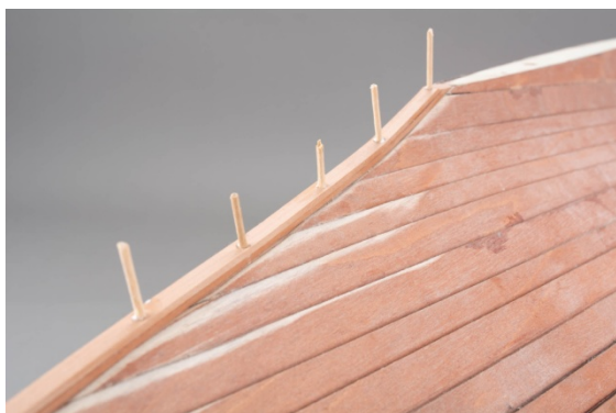
Fig.: Closing of the screw holes
