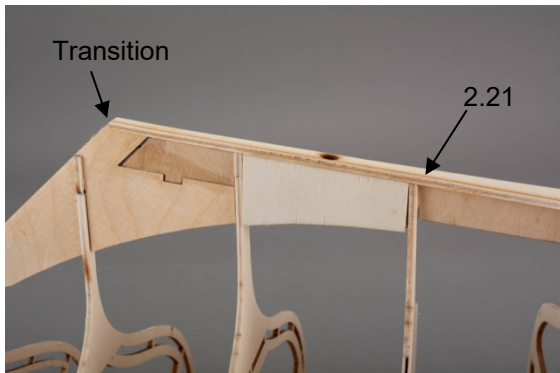
Fig.: Aligning and gluing on the keelboard, keel bolt at the rear
