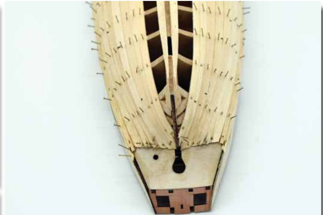
Planking at the stern - Still very little tapering was required for the stern
