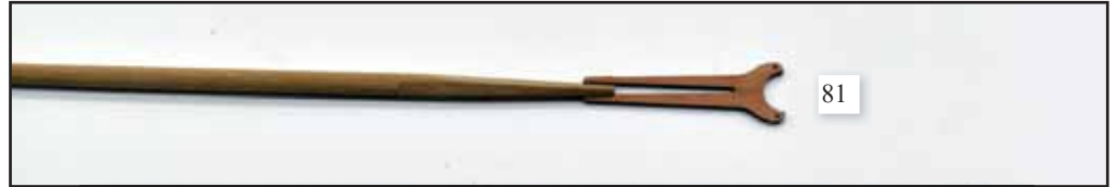
132. Shape the driver boom and gaff yards as per the plans, and add the jaws to the ends
