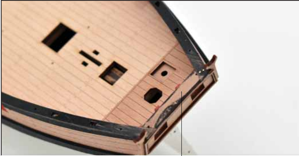
79. Add the stern transom gunwale (123). This will need a little filing in order to get it to fit in between the aft parts of the side gunwales. Once in place, paint black.
