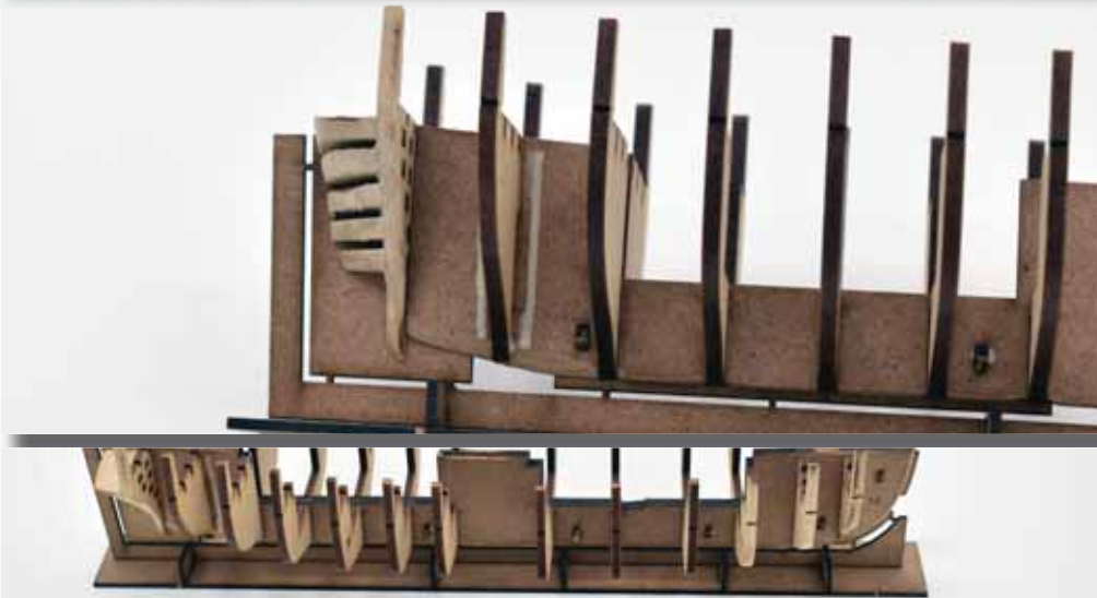
13. Remove the lower deck (25) from the 2mm MDF sheet, ready for slotting into place
