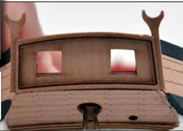
76. Remove the stern transom framing (83a) from the 0.8mm wood sheet and glue in place, as shown, You can use either PVA wood glue and pin in place or cyano glue.
