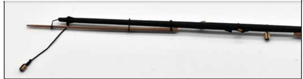
The main yard now with all its various blocks attached. Once the blocks have been fitted, add the stunsail booms (below). The inner ends can be secured by simply adding 0.25mm black thread, tied around the yards two or three times.
