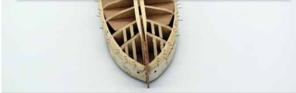
Planking progress with three planks per side done. For the prototype, one plank per side is laid.
