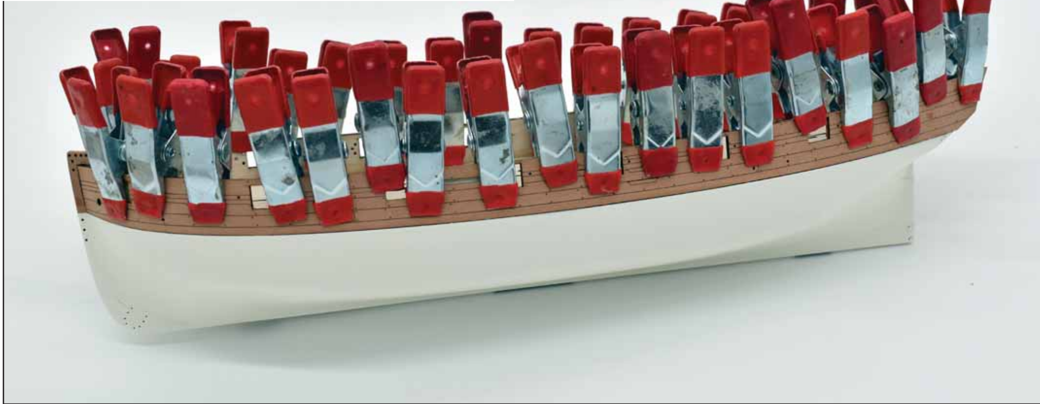
60. Now that all of the 'messy' work has been done, the outer bulwark patterns can now be glued into place. No pins were used, just claps. As with almost all wood to wood fixing, PVA wood glue was used. This was brushed onto the ply side, and the wood engraved bulwark placed and clamped in place, as shown.
