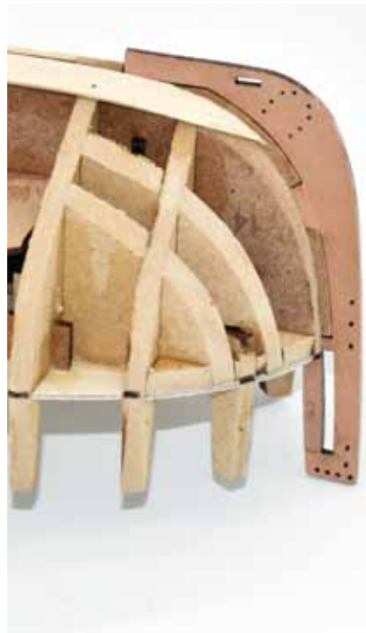
42. Glue the prow in place using PVA wood glue
