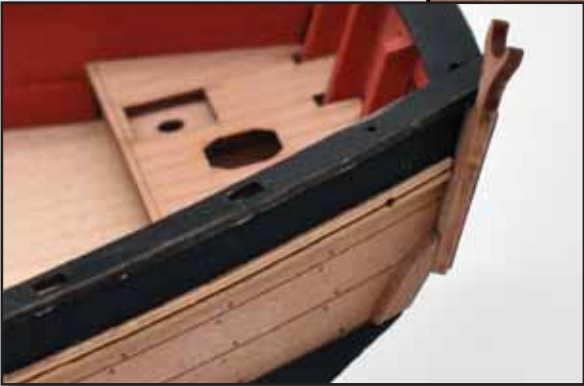
82. Remove the stern side counter timbers (74) and glue in place to the position shown
