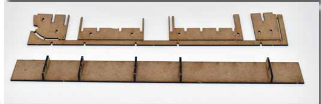
2. Glue the keel supports into the slots in the base. Remove the main keel (20) from the 2mm MDF sheet. Be careful when handling this, as it is in 4 sections, and held together on its jig to keep the sections spaced correctly until built up
