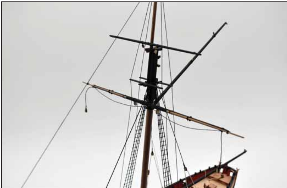
147. Two pictures showing the 2 breast backstays per side. The lower ends are secured around the first and last lower deadeye for the shrouds, and then taken up through the hole located near the end cross-trees and then tied to the topmast head, at the cleat positions.
