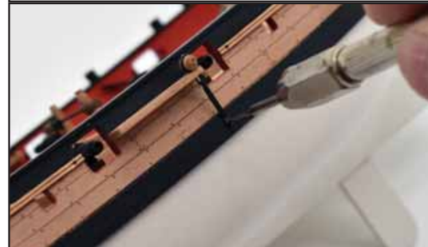
112. Push/drop the chainplate through the slot in the channel and drill a 0.6mm hole to secure the lower chainplate with a brass pin. The pin can then be pushed all the way in to secure the chainplate.
