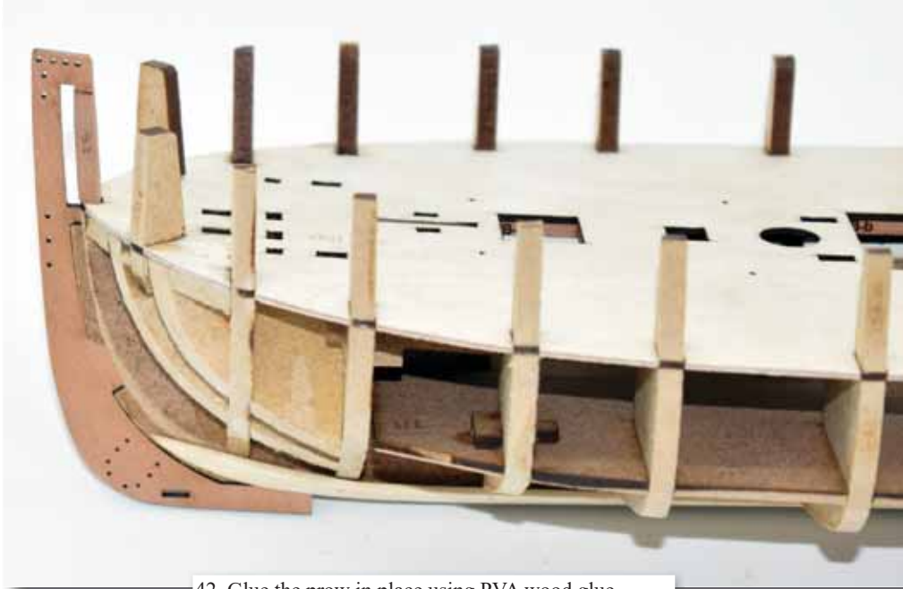
42. Glue the prow in place using PVA wood glue
