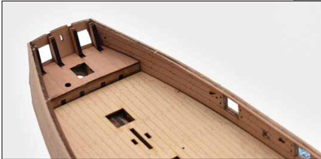
Inner bulwarks in place. Note the slight gap between the bottom edge of the bulwarks and deck.
