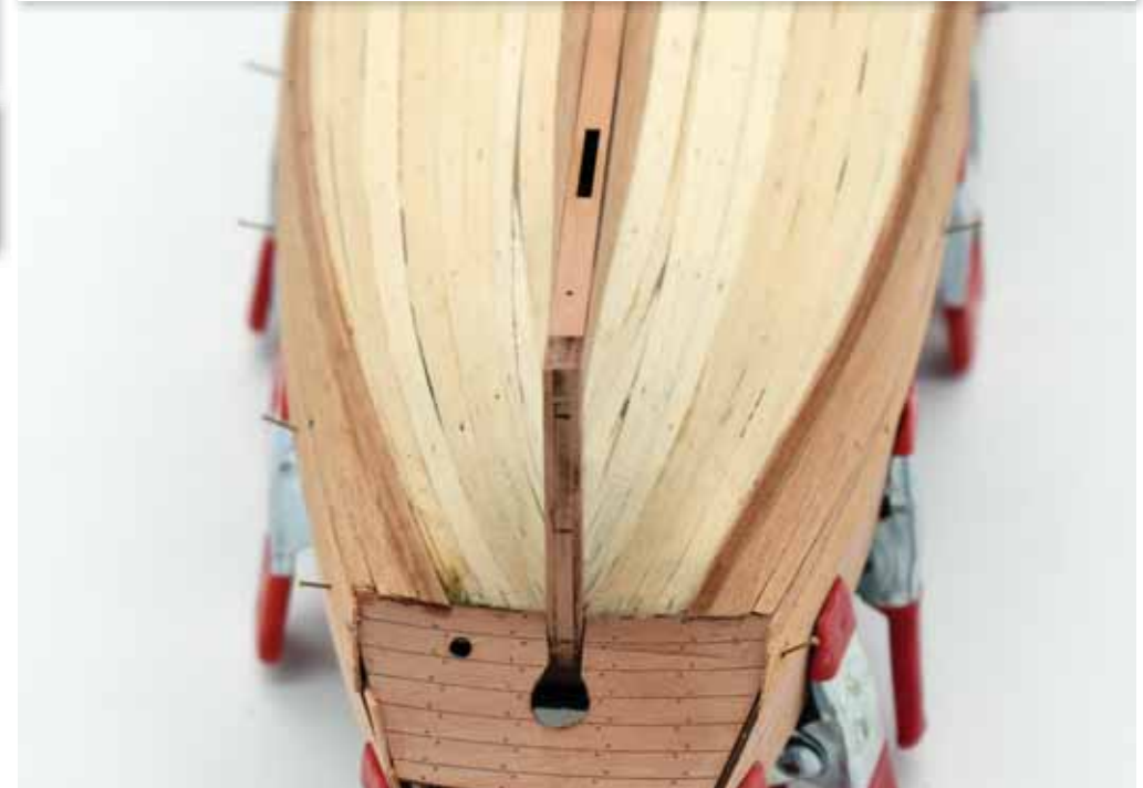
Planking progress at bow (above) and stern (below). If you do not get the end planks at the stern perfectly butted up against the stern counter, do not worry too much, as this line is covered by stern counter rails (124 and 125)
