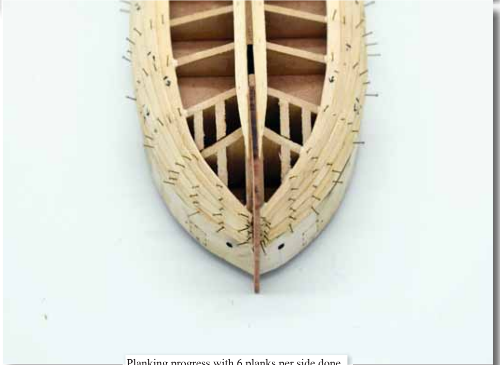
Planking progress with 6 planks per side done
