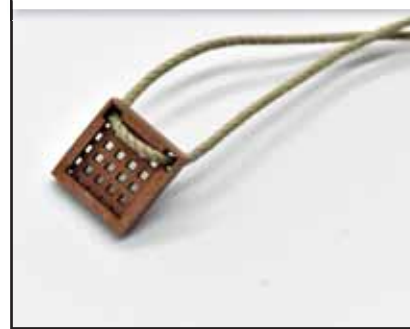
117. Thread the anchor hawse rope through the holes in the fore gratings, as shown, and then glue the gratings in place.
