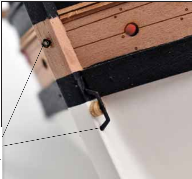
113. Once all chainplates have been fixed in place, carefully paint the pin heads black
