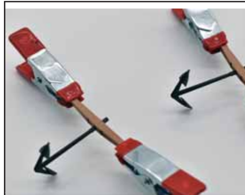
118. Before gluing the halves of the anchor stocks together, test fit the anchor shaft between them and if necessary, deepen the engraved area a little when the anchor sits comfortably within, remove the anchor and glue the stock halves together.
