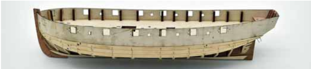
Planking progress with three planks per side done. For the prototype, one plank per side is laid.
