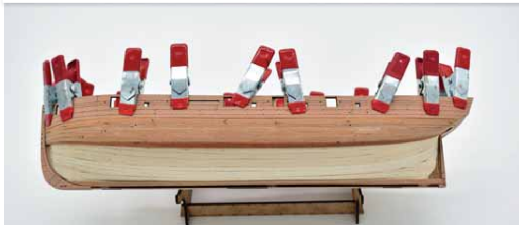
As with the first planking, the planks require tapering at the front (as shown above) Below - The first 4 planks laid.
