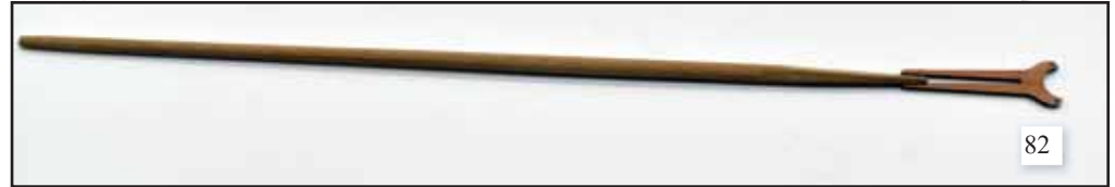
132. Shape the driver boom and gaff yards as per the plans, and add the jaws to the ends
